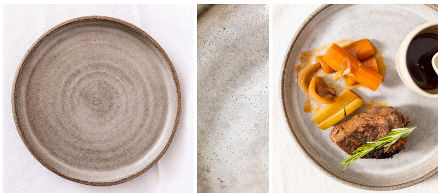
Figure 48. The symmetrically correct plate with the glitch in the glazing where bubbles appear on the surface of the plate. Photographs by Kristi Palm Anis
